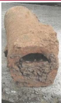
Figure 22. Silted clay drain
