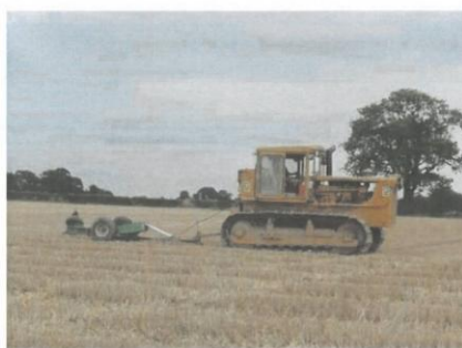
Figure 30. Installing mole drains
