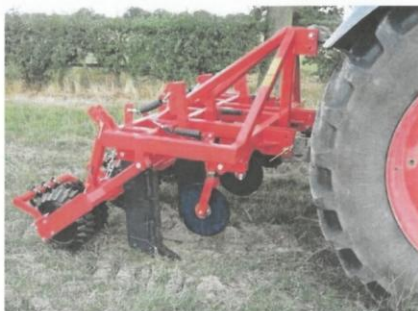
Figure 11. Topsoil loosener for grassland
